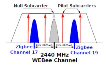
Central frequency of a WEBee channel is set so there are ZigBee channels which do not overlap with the Null subcarrier
