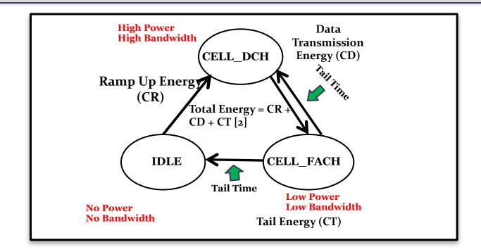
**Total Energy Consumption = CR + CD + CT**, where CR is the ramp up energy (**IDLE to CELL DCH**), CD is the data transmission energy, and CT is the tail energy (in CELL FACH).
